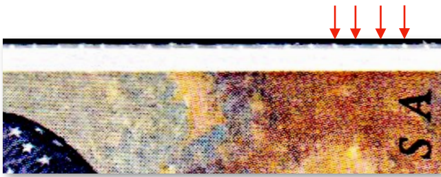
Figure 3. Tiny bridges hold the BCA coils together in a stick. Coils from the inner rows of the web have the bridges on top and bottom. The coils from the outer edges of the web have bridges either on top or the bottom. These are easier to see on stamps that are off their backing
