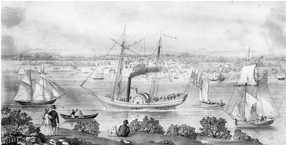
Page 1. Walk-in-the-Water at Detroit, 1820. This contemporaneous sketch by George H. Whistler appears to depict many details of the vessel accurately, such as the transom stern, raised quarterdeck and twin (black) stripes along the hull.
