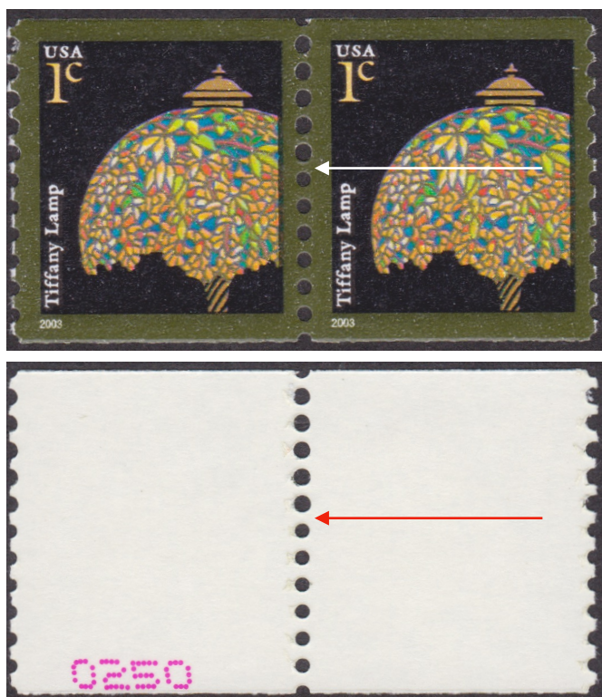
Figure 5. 1¢ Tiffany Lamp, Scott 3758, from a 3,000-stamp roll. Large holes above small holes, with the change occurring at the arrow. With the dark design, the difference is most easily seen from the back. Three sets of pins were used to perf this web, overlapping at two points. Only coils at one or both of the overlaps would show the change in perforation diameter; so these are not common.
